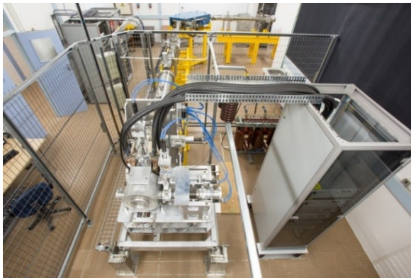
Figure 2: The LERIB test-bench contains a target/ion source (foreground) on a high-voltage platform, and a beamline with an analysing magnet (background).
