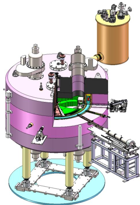
Figure 7: The preliminary structure of cyclotron.
