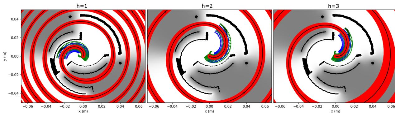
Figure 1: The new central region of the K130 with all three harmonics. The beam depicted in red has a geometrical envelope emittance of  $100 \pi$  mm mrad at the inflector entrance and all particles are injected at phase  $0^\circ$ . The black line is the reference orbit with particle location at the time of dee voltage maxima marked with a cross.
