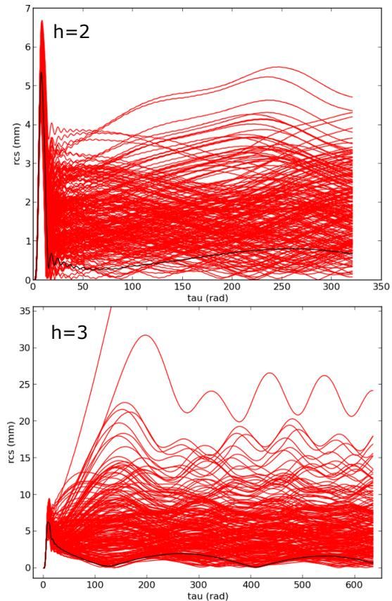
Figure 3: Centering of the full injected beam for  $h = 2$  and  $h = 3$ . The reference orbit is drawn in black.
