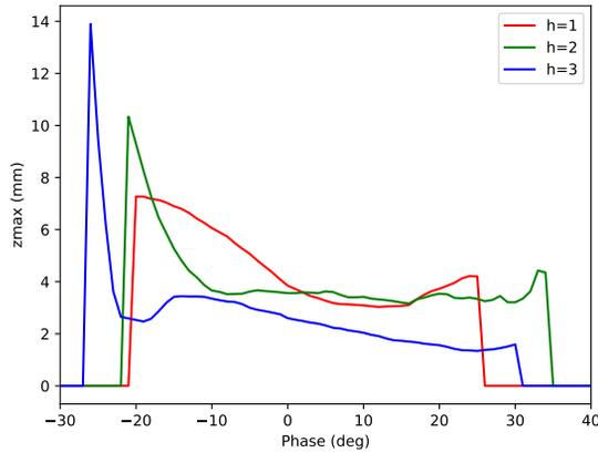
Figure 2: The maximum vertical position of a particle launched at the end of the inflector off the midplane, at  $z = 1$  mm as a function of the starting phase. A non-zero value is shown only for particles reaching the extraction. Zero phase refers to the phase producing the highest energy gain per turn for a particle launched on the midplane.
