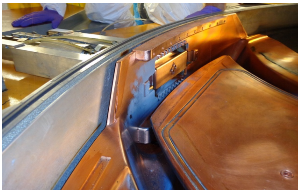
Figure 4: Cadmium deposition on RF system after outgassing of the mobile capacitor brazing.
