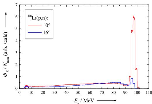
Figure 3: Neutron spectra (measured by time-of-flight) from 100 MeV protons on a 6 mm  ${}^{\text{nat}}\text{Li}$  target.
