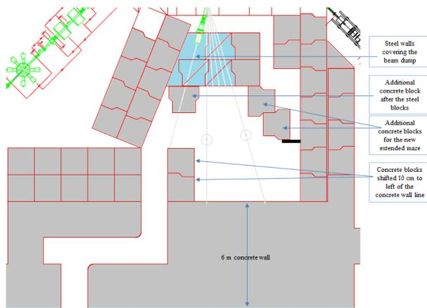
Figure 7: The proposed new configuration of the iThemba LABS neutron beam vault.
