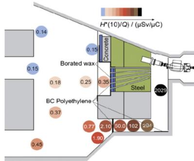
Figure 6: Ambient dose equivalent,  $H^*(10)$ , at various locations within the fast neutron beam vault at iThemba LABS measured for a 200 MeV proton beam on a 6 mm Li target [8].
