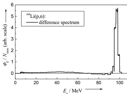
Figure 4: Difference spectrum obtained by subtracting the 16° spectrum from the 0° spectrum.
