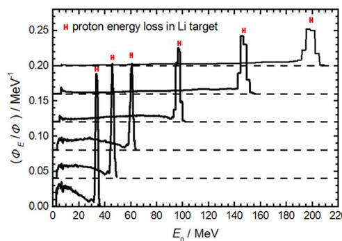
Figure 5: Normalised neutron spectra from Li targets at various energies produced at iThemba LABS [9].
