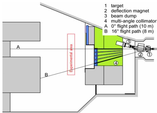
Figure 2: Layout of the fast neutron beam facility at iThemba LABS.
