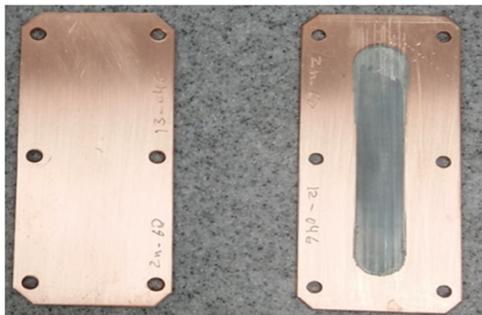
Figure 5: The copper target before and after being coated with the Zn-68.
