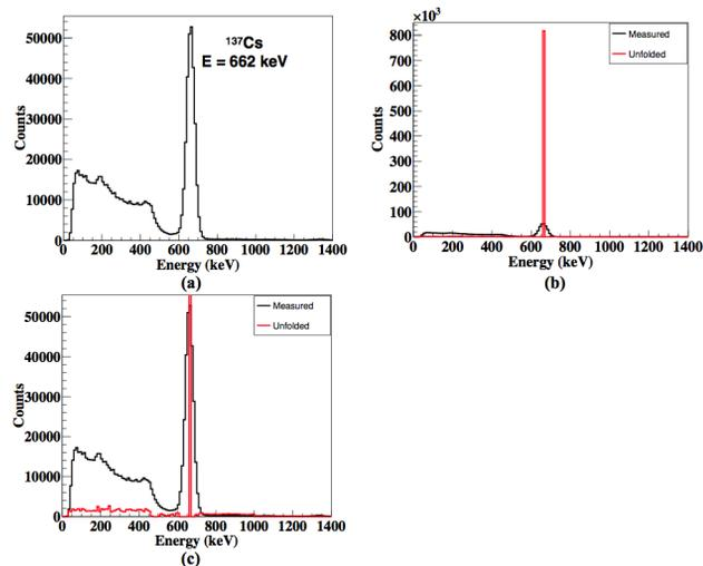
Figure 4: (a) The measured energy spectrum of  $^{137}\text{Cs}$  (overlaid as black histogram) (b) The deconvoluted spectrum (overlaid as red histogram) using matrix inversion method.
