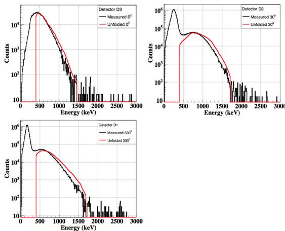
Figure 6: Deconvoluted energy spectra at angles  $0^\circ$  (D3),  $30^\circ$  (D2) and  $330^\circ$  (D1) respectively obtained after unfolding.
