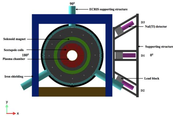
Figure 1: The three NaI(Tl) scintillation detectors at the center of the ECR ion source.
