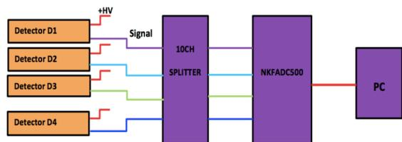
Figure 3: Schematic of an electronic illustration showing the signal from each detector was fed to the splitting module and then to other electronic devices.
