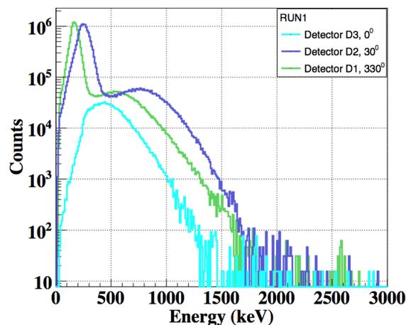
Figure 5: Bremsstrahlung photons energy intensity measured in three angles for detectors D1, D2 and D3.
