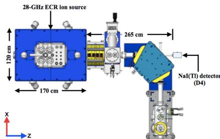
Figure 2: Detector D4 at the view port. The D4 detector was used to monitor a possible variation in ECR plasma intensities throughout the measurements.
