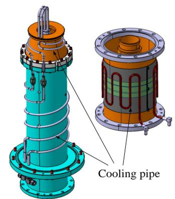
Figure 3: Cooling pipes on RF window and coupling.
