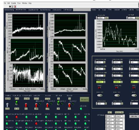
Figure 2: The interface of LLRF system for RF conditioning.
