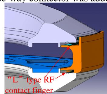
Figure 4: "L" type RF contact finger for Dee
