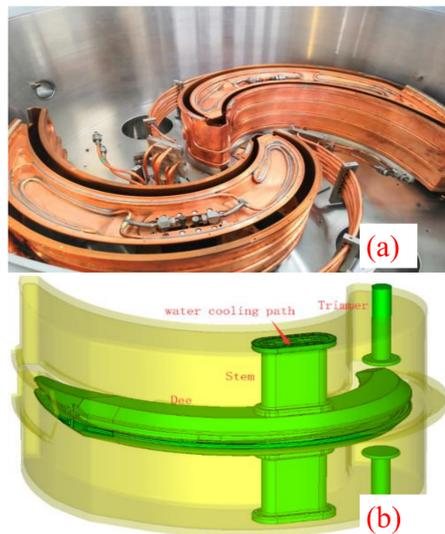
Figure 1: Layout of RF cavity.
